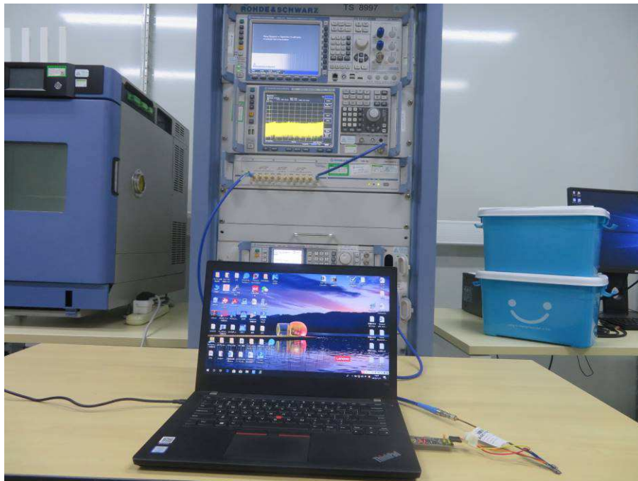
Photograph 1: Set-up for Radio Spectrum Test
