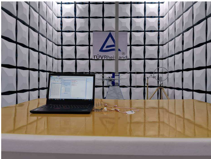
Photograph 2: Set-up for Radiated Spurious Emission, 30MHz ~ 1GHz
