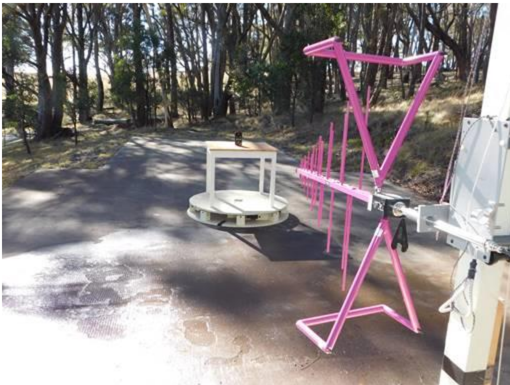
Figure 2: EUT, at OATS, radiated emissions testing.
