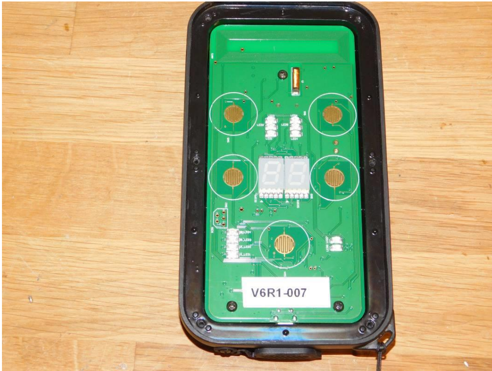
Figure 1: EUT, front view with top cover removed.
