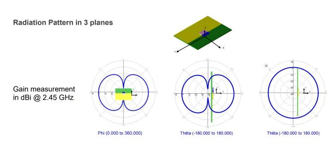
The antenna Gain max is 0.6dBi
