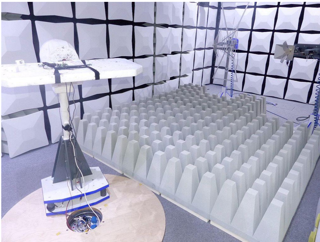
Photo 3: Test setup for radiated measurements (Enclosure, fully-anechoic chamber, 1-26 GHz intentional radiator §15 / 30 MHz – 10/20 GHz §22/24/27)
