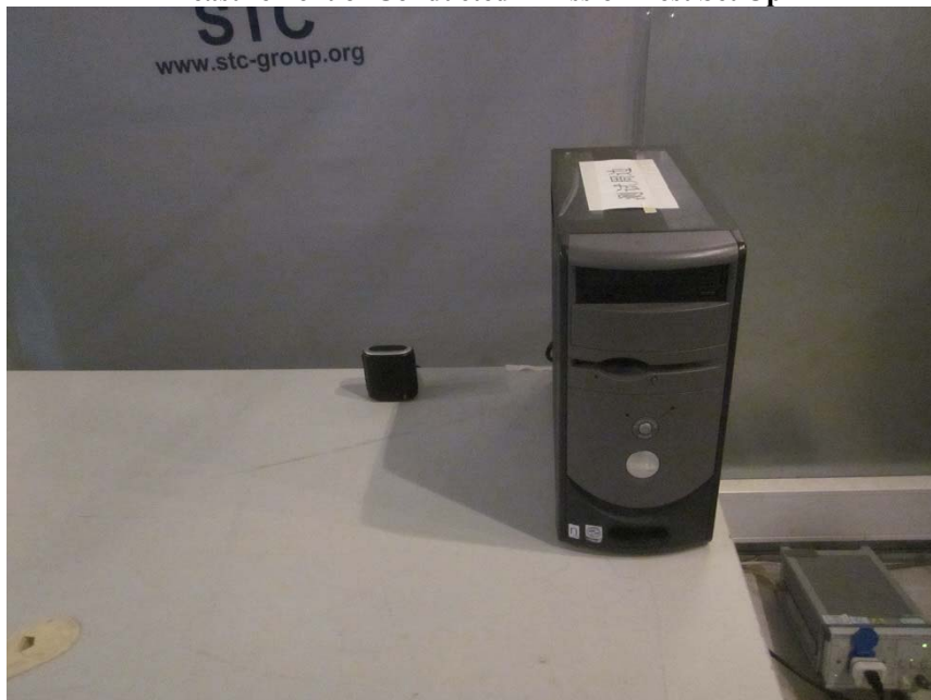
Measurement of Conducted Emission Test Set Up
