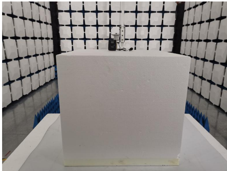
Above 1GHz for radiated emission test setup
