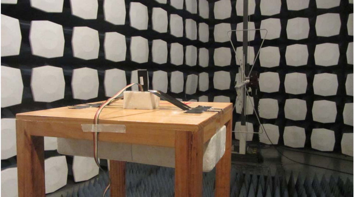
Picture 2: Radiated Spurious Emissions Test setup
