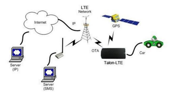
This LTE product is designed based on the Sequans Communications US130Q LTE E-UTRA or VZ120Q (4G LTE CAT 1, wireless data/SQN3223) baseband module, which includes an ARM CPU, 4M serial flash, LTE\_B2&B4&B12 RF transceiver, and triple-band RF front end circuit.
