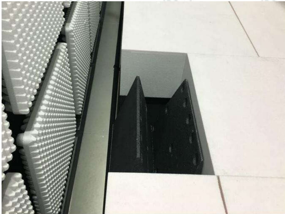
Radiated spurious emission Test Setup-4(Above 1GHz) There is absorber on the ground floor
