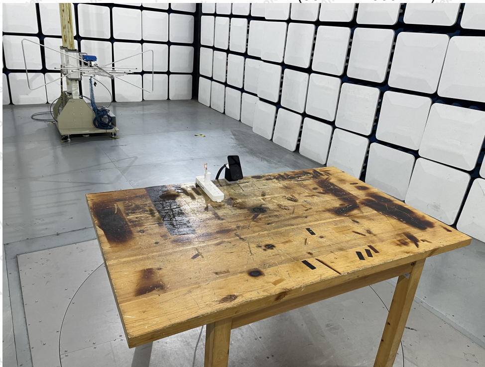
Photo of Radiation Emission Test (30MHz~1000MHz)
