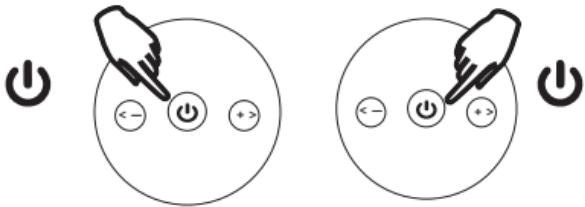
1. Press and hold the Power buttons on each speaker for 2-3 seconds to turn them ON. Wait approximately 10 seconds and your two speakers will pair together. Restart both speakers if they aren't pairing together after an extended period of time.
