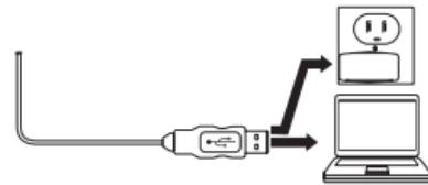
3. Insert the USB charging cable's standard USB plug into the USB port of a computer or suitable 5V 1A USB charging adapter.
