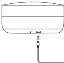
2. Insert the USB charging cable's Micro USB plug into the charging port on your speaker.
