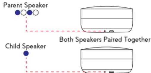
2. Once your two speakers are paired together, the parent speaker's indicator light will turn blue and flash. The child speaker's indicator light will turn blue and shine steadily. Note that buttons on both speakers should be functional, not just the master speaker.
