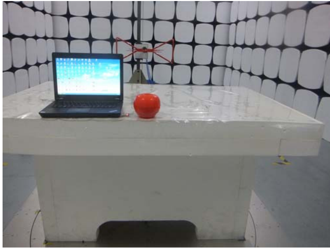
Radiated Spurious Emissions Test Setup Below 1GHz
