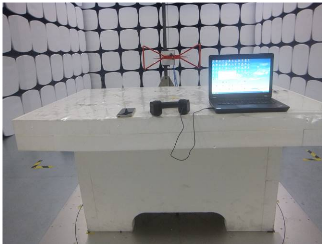
Radiated Spurious Emissions Test Setup Below 1GHz
