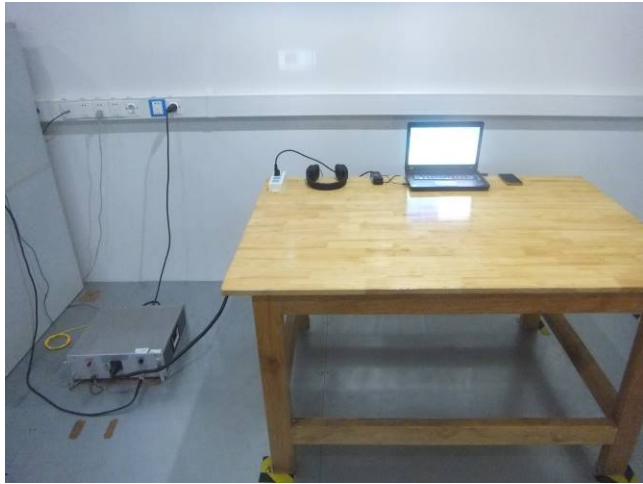
Conducted Emissions Test Setup Front View
