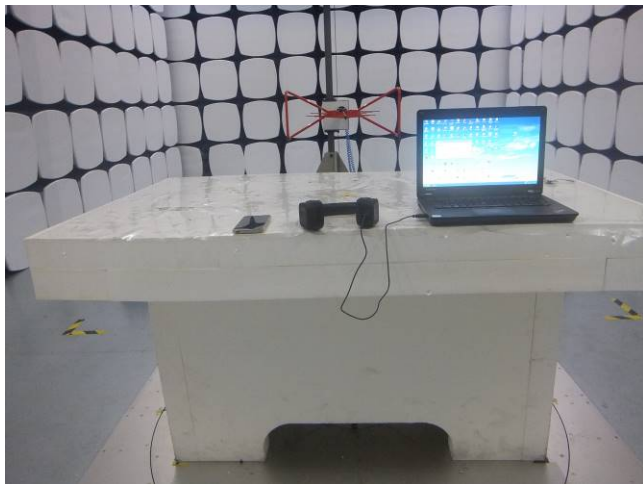
Radiated Spurious Emissions Test Setup Below 1GHz
