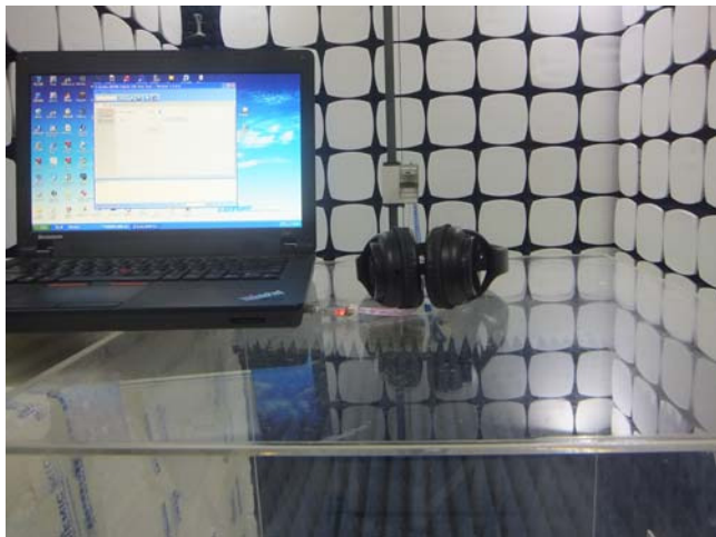
Radiated Spurious Emissions Test Above 1GHz
