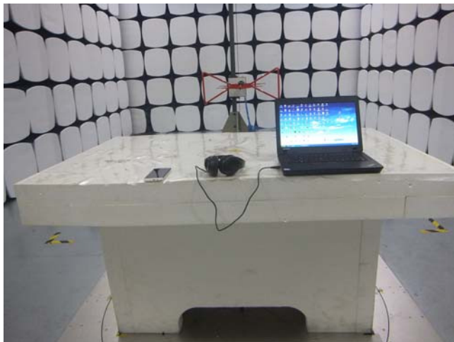
Radiated Spurious Emissions Test Setup Below 1GHz
