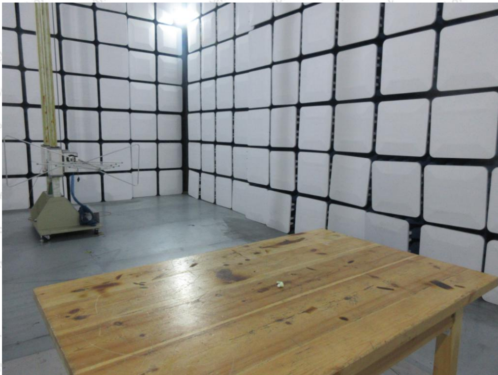
Photo of Radiation Emission Test
