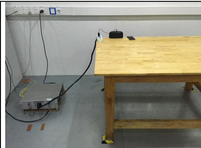
Conducted Emissions Test Setup Front View
