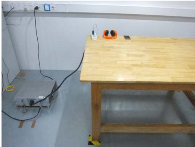
Conducted Emissions Test Setup – Front View
