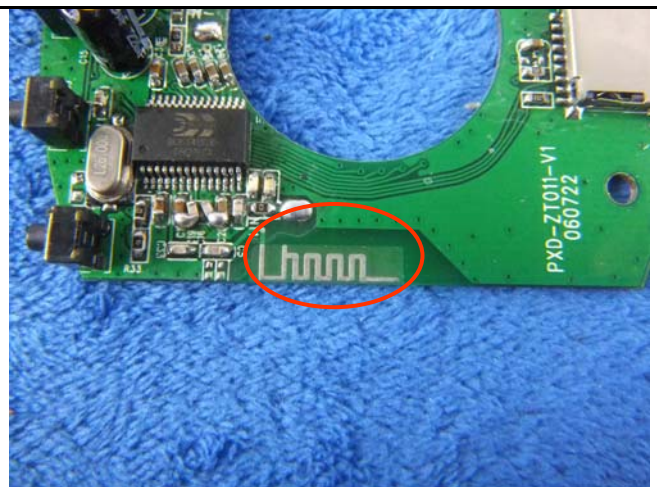
BT - Antenna View
