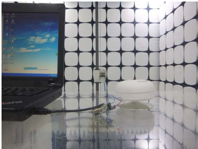
Radiated Spurious Emissions Test Above 1GHz
