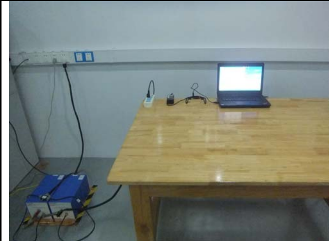
Conducted Emissions Test Setup – Front View
