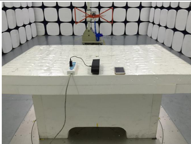
Radiated Emissions Test Setup Below 1GHz
