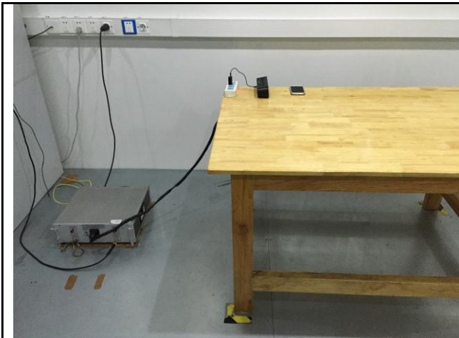
Conducted Emissions Test Setup Front View
