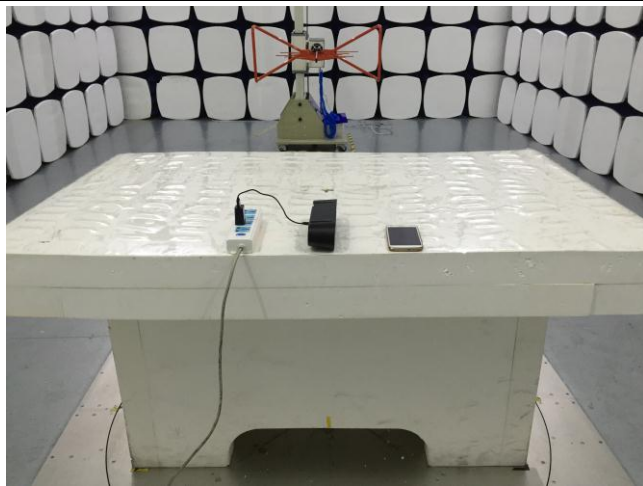
Radiated Emissions Test Setup Below 1GHz
