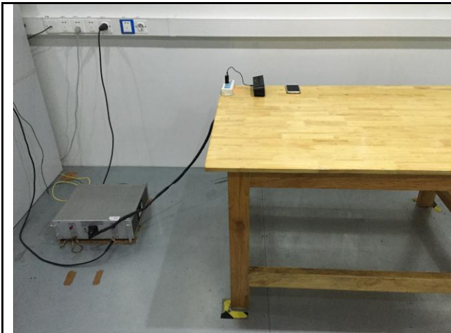
Conducted Emissions Test Setup Front View
