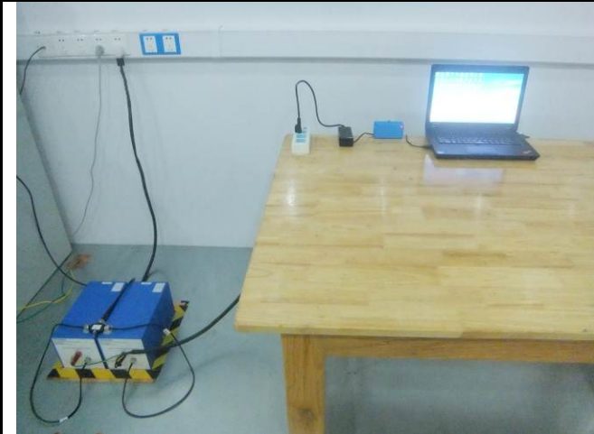
Conducted Emissions Test Setup Front View
