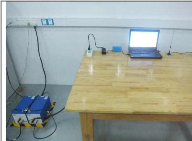
Conducted Emissions Test Setup Front View
