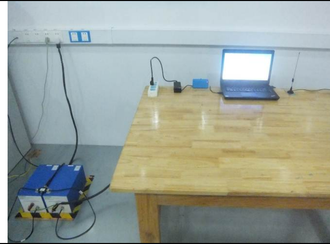
Conducted Emissions Test Setup Front View
