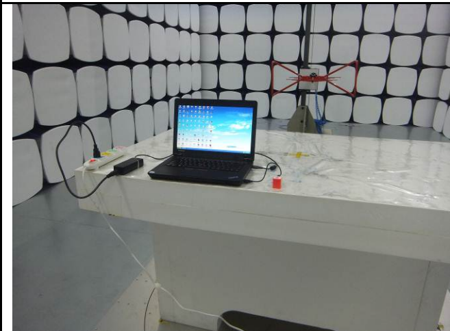
Conducted Emissions Test Setup Front View
