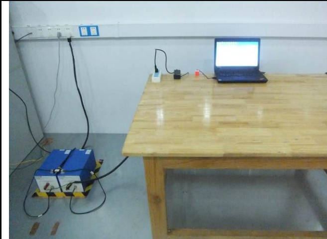
Conducted Emissions Test Setup Front View
