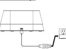
Use the included USB-C cable to power your charging station. 1.Insert the USB-C connector into the USB-C port on your charging station.
