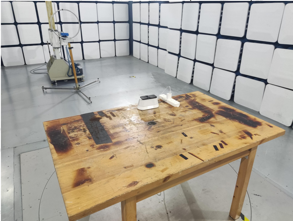
Photo of Radiation Emission Test (below 30MHz)
