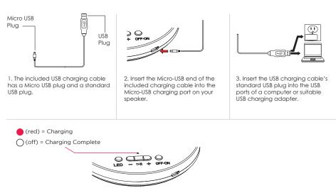
4. The LED indicator light turns red while the speaker is charging. It turns off once charging is complete.
