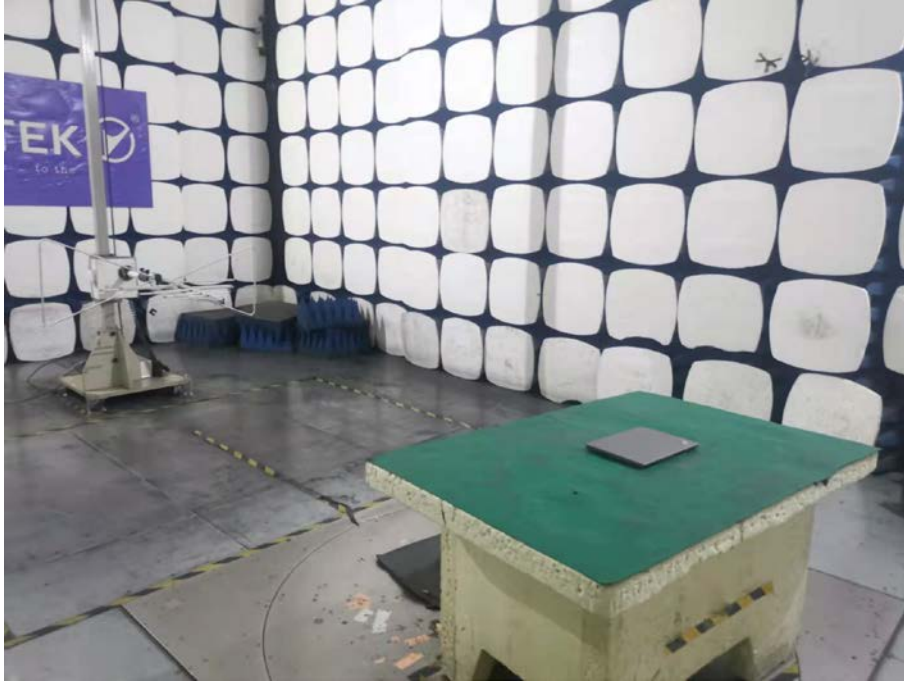
Spurious Emission Test Setup (Above 1GHz)
