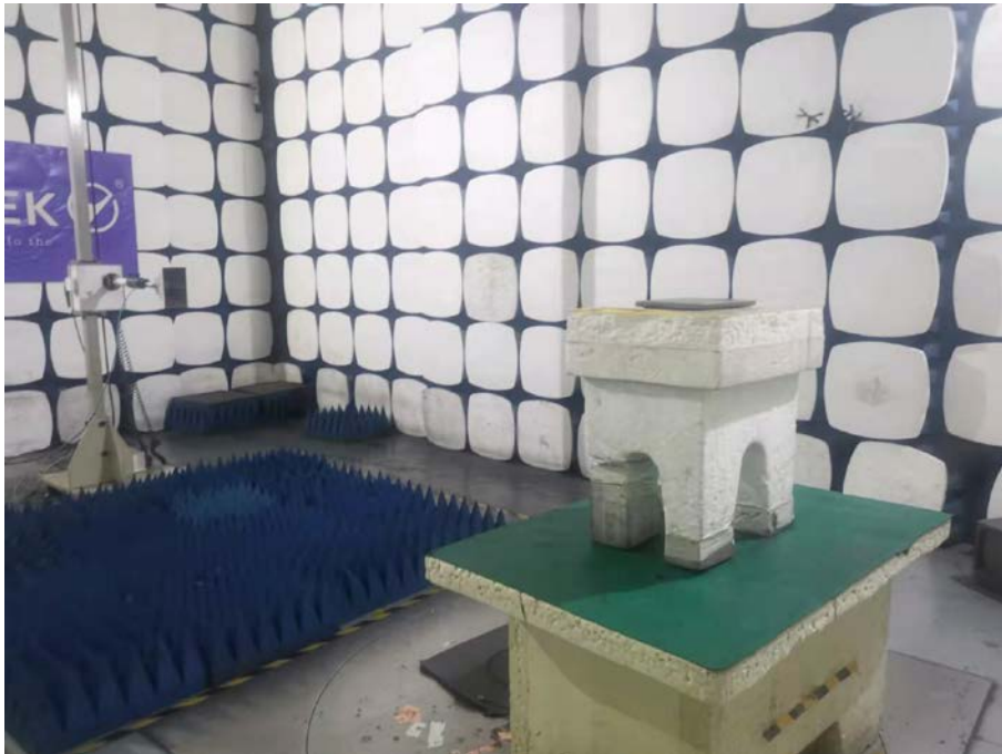
Spurious Emission Test Setup (Above 1GHz)
