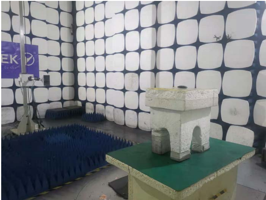
Spurious Emission Test Setup (Above 1GHz)
