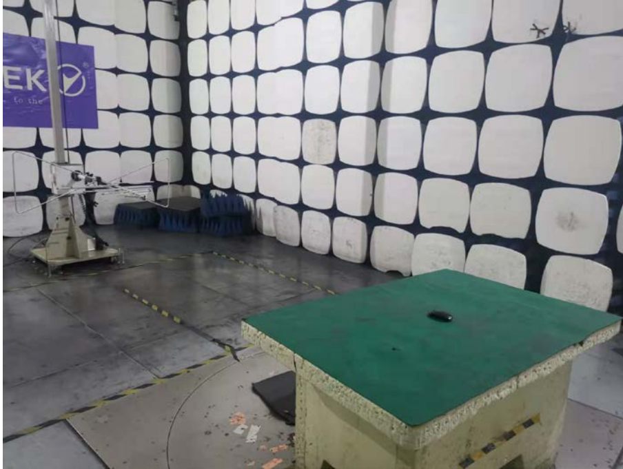
Spurious Emission Test Setup (Above 1GHz)
