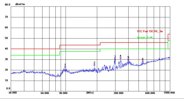
Site #2 3m Anechoic Chamber Polarization: Horizontal Temperature: 25.3(C) Humidity: 51 %
