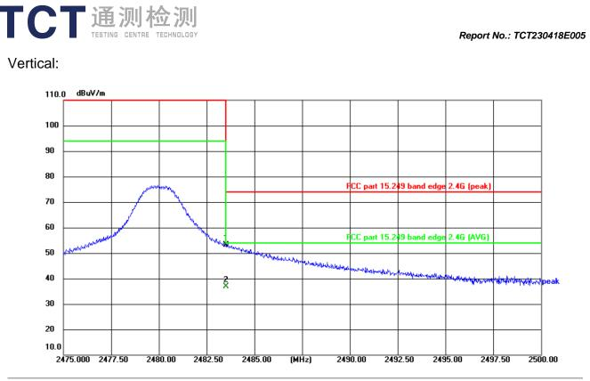
Site: #3 3m Anechoic Chamber Polarization: Vertical Temperature: 24(°C) Humidity: 52 %
