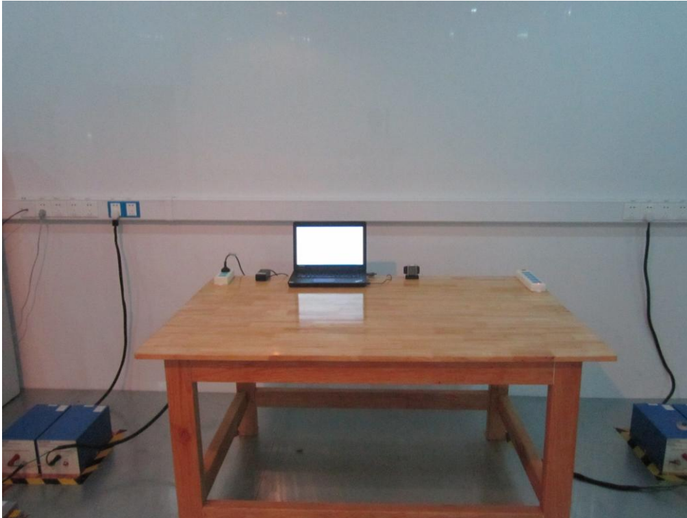
Conducted Emissions Test Setup Front View
