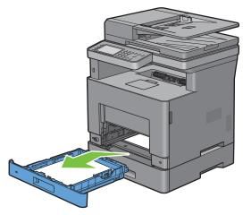
**5** Pull the optional 550-sheet feeder from the printer about 200 mm.
