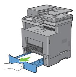
**6** Hold the optional 550-sheet feeder with both hands, and remove it from the printer.
