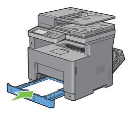
8 Insert the MPF into the printer.
