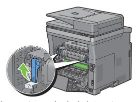
3 If the document is jammed under the fusing unit, remove the jammed document from under the fusing unit.
