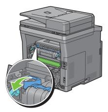
**5** Remove the jammed document from above the fusing unit.
