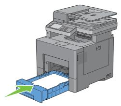
**12** Insert the MPF into the printer.
