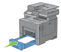
7 Insert the MPF into the printer.
