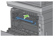
**6** Press down the levers on both sides of the fusing unit, and then close the rear cover.
