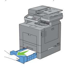
**2** Hold the optional 550-sheet feeder with both hands, and remove it from the printer.
