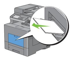
**2** Grasp both sides of the MPF, and then pull it out of the printer.
