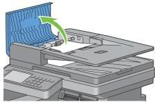
Lift the release lever 90 degrees and remove the jammed document by carefully pulling it to the right.
