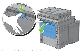
**2** Lift the levers on both sides of the fusing unit.
