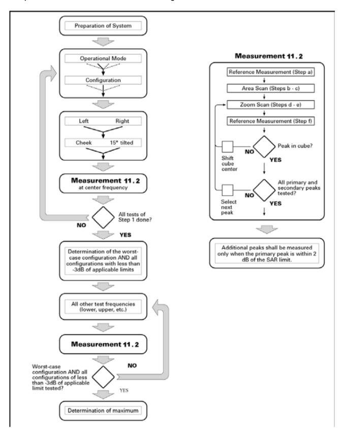
Picture 10.1 Block diagram of the tests to be performed
