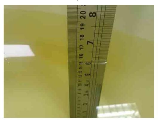
Liquid depth in the Flat Phantom (2450MHz)
