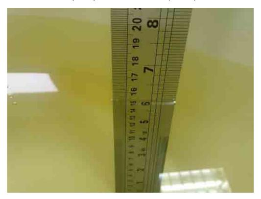
Liquid depth in the Flat Phantom (1900MHz)
