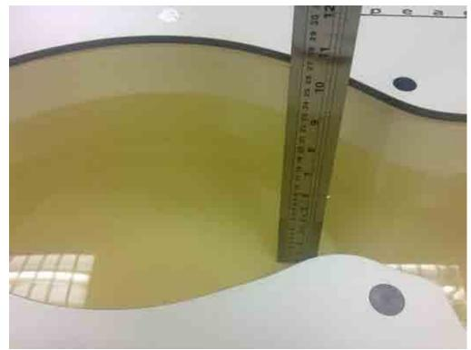
Liquid depth in the Flat Phantom (835MHz)
