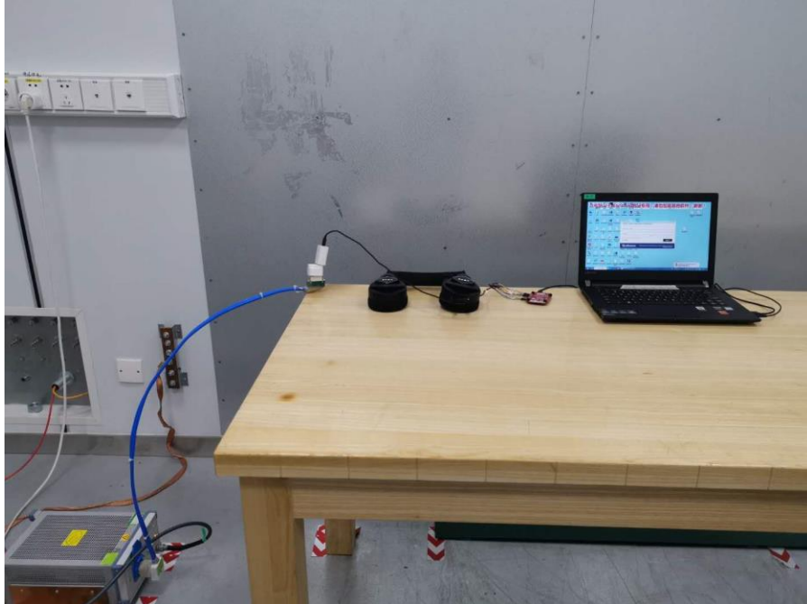
POWERLINE CONDUCTED EMISSIONS MEASUREMENT SETUP
