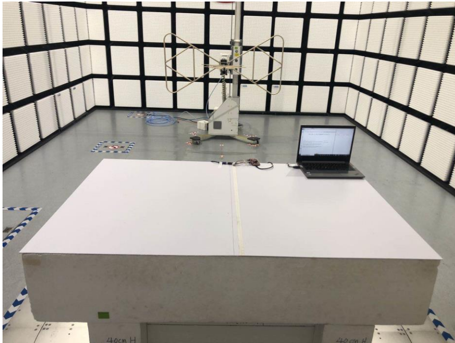
RADIATED RF MEASUREMENT SETUP (30MHz~1GHz)
