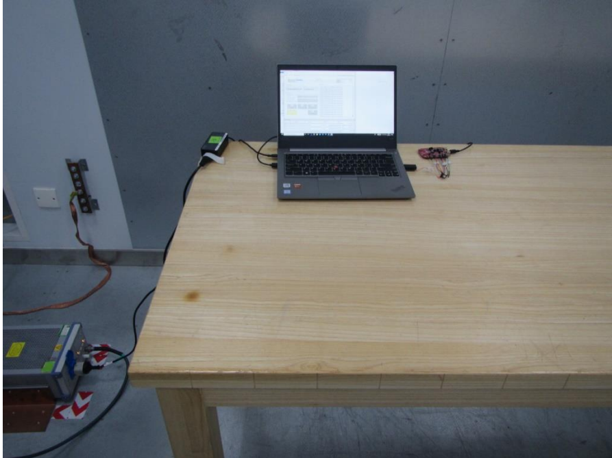
POWERLINE CONDUCTED EMISSIONS MEASUREMENT SETUP
