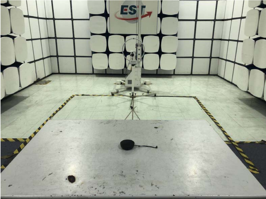
Radiated Test (Below 30MHz)
