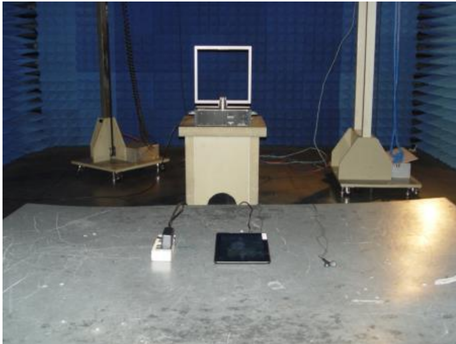
Photograph 2: Set-up for Radiated Spurious Emissions (30MHz-1GHz)
