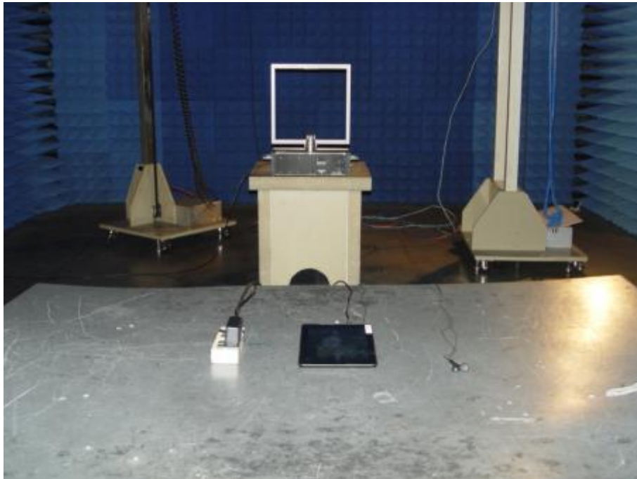
Photograph 2: Set-up for Radiated Spurious Emissions (30MHz-1GHz)
