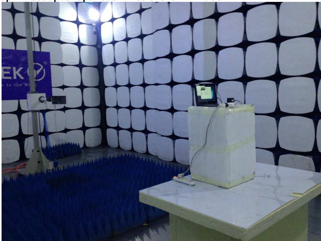
Photograph 4: Set-up for Spurious Emissions for 1 - 26.5GHz
