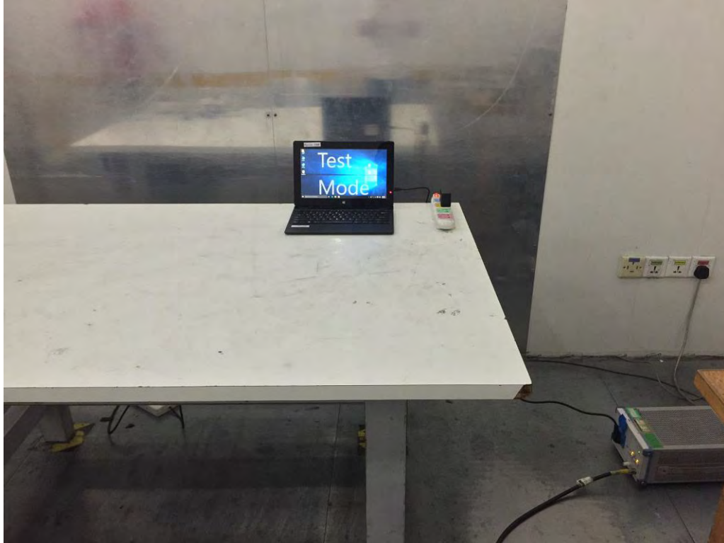
Photograph 2: Set-up for Spurious Emissions for below 30MHz
