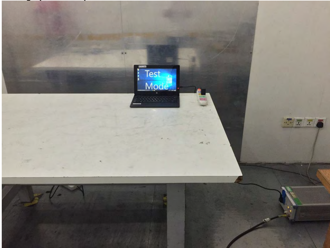
Photograph 1: Set-up for Conducted Emission
