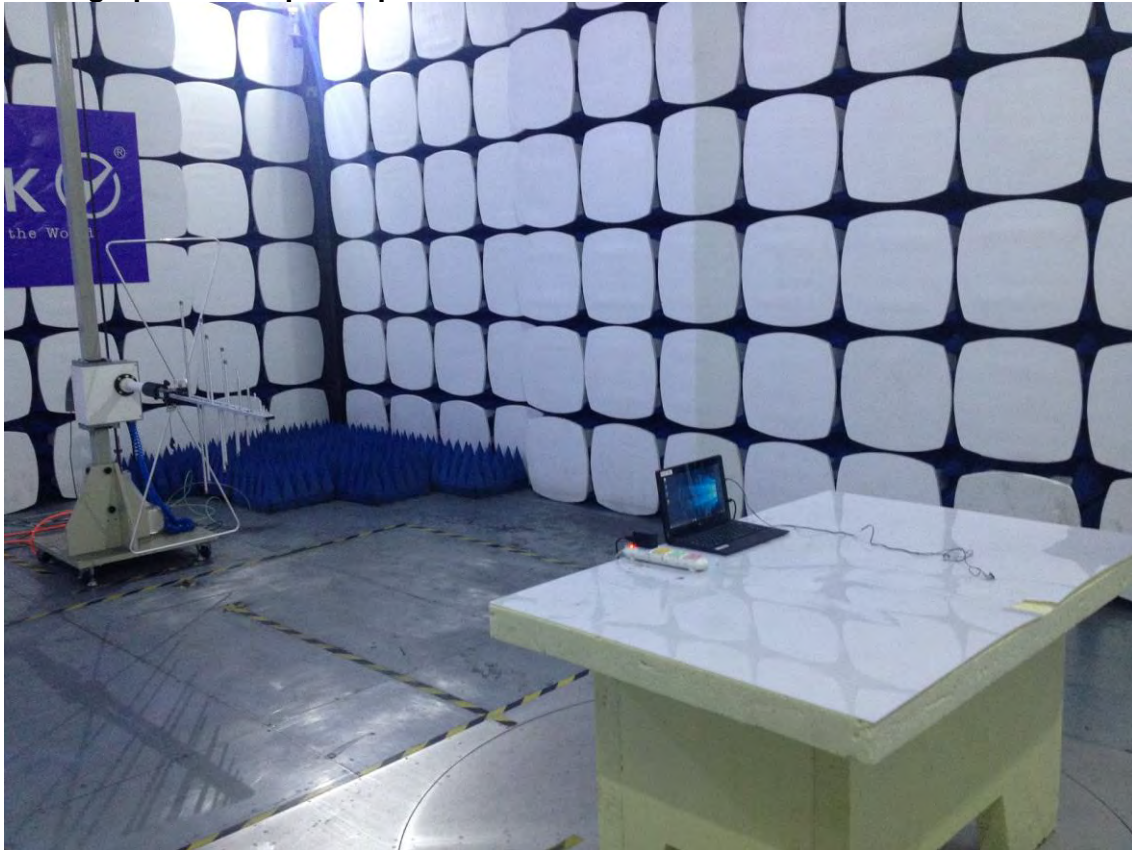
Photograph 3: Set-up for Spurious Emissions for 30 - 1000MHz
