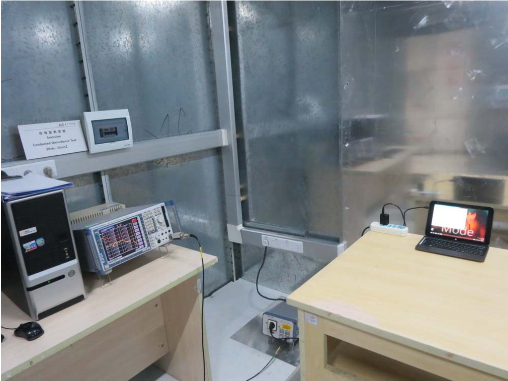
FCC RADIATED EMISSION TEST SETUP
