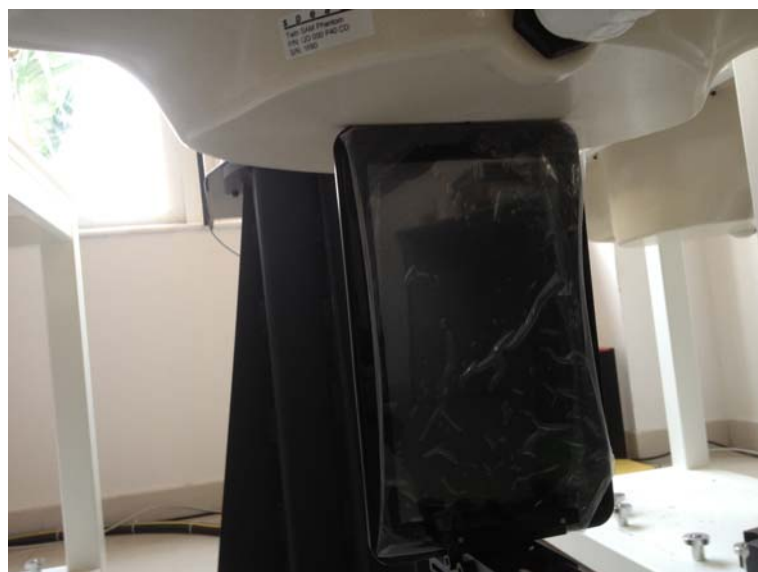
0mm Body-worn Bottom Side Setup Photo
