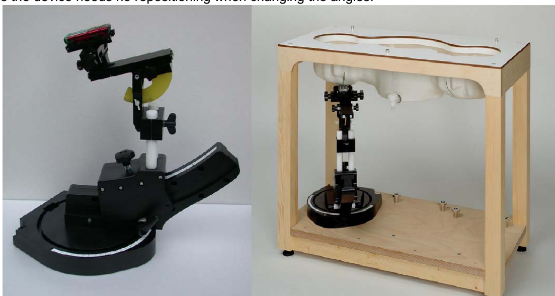
Device holder supplied by SPEAG
