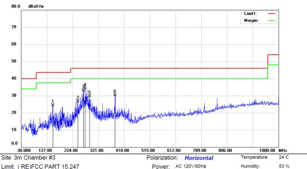
Limit: (RE)FCC PART 15.247 Mode: 802.11b TX Channel6
