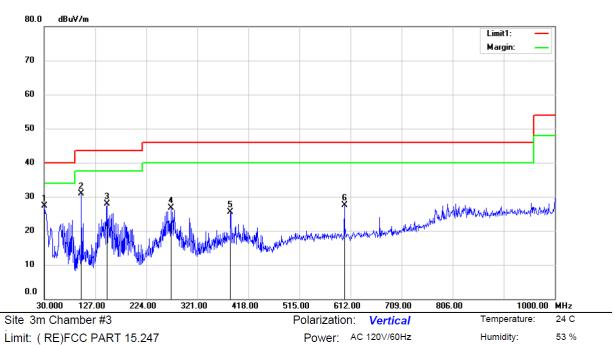
Limit: ( RE)FCC PART 15.247 Mode: 802.11b TX Channel1
