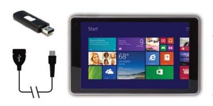
Insert a USB flash drive or external hard drive into the USB port using the included transfer cable. In addition, you can add an external mouse, connect a keyboard, or other USB compatible device.
