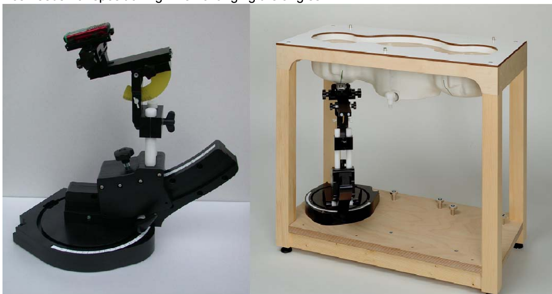
Device holder supplied by SPEAG
